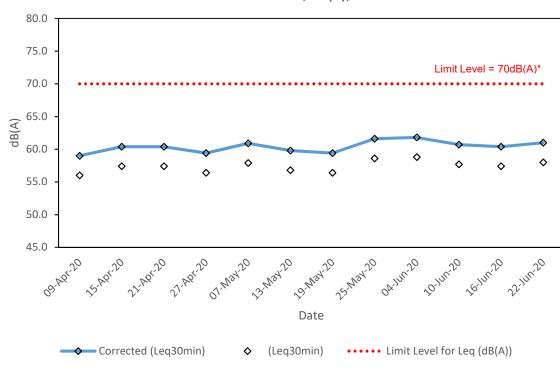
Noise Level for 30 min, dB(A), at NM1A
